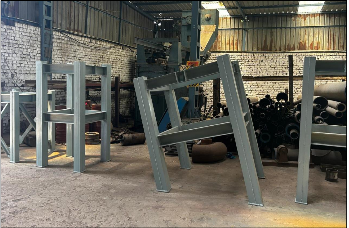
PRODUCT: STRUCTURE (PIPE SUPPORT) END USER:
